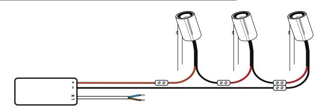
TYPICAL WIRING. NOTE SERIES CONNECTION - INTO POSITIVE, OUT OF NEGATIVE INTO POSITIVE ETC. Easy connection boards are available as an alternative.
